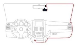
The camera should be positioned near the rear view mirror, in order to have a good front view. The best position is towards the passenger side, as shown, so as not to obstruct the driver's view.
